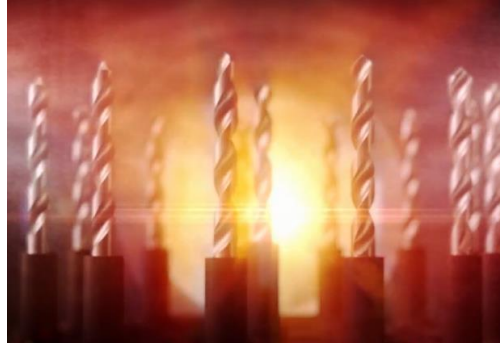
Drills getting coated in a PVD vacuum chamber
