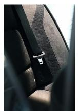
**Caption:** In accidents, the number one lifesaver is not the vehicle's body work or the airbag, but the seat belt. It holds the vehicle occupants firmly in position and thus enables other protective technologies to unfold their full function.
