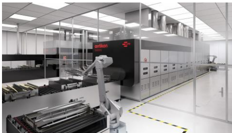
Fig. 9: INUBIA I (ePD): Integrated equipment for the metallisation of plastics (ePD).
