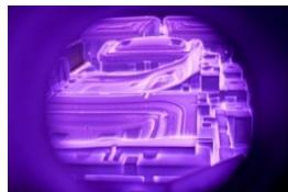
A look inside the vacuum chamber, the core of PPD™ technology: Large automotive forming tools are repeatedly coated with pulsed plasma. No toxic waste products are generated.
