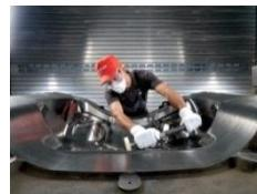
An Oerlikon Balzers employee checks the surface finishing and conducts quality control on coated forming tools.
