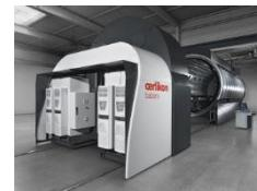
With a loading capacity of 10x3 meters and 40 metric tons, PPD™ technology can even coat the automotive industry's largest press tools.
