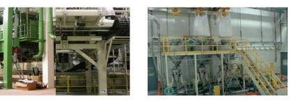
Airlaid lines are for the production of absorbent core materials, wipes, napkins and table tops.
