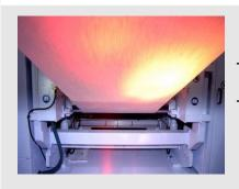
The world's largest spunlaid spinning system – from Oerlikon Neumag – produces non-woven textiles up to 7 meters (23 feet) wide.
