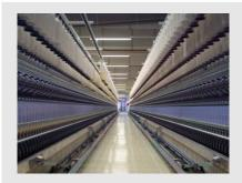
The world's largest ring spinning system – from Oerlikon Schlafhorst – has up to 1,680 spinning points and is over 70 meters (230 feet)
