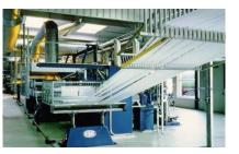
Spunlaid lines up to 7m wide have broad applications, from hygiene to technical. Meltblown lines are for filtration and barrier applications.
