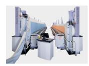
Twisting and cabling machines for high performance varns in tires and different technical applications
