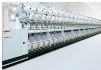
Twisting and cabling machines to manufacture BCF-carpet yarns for design variety, long-life cycle and comfortable touch
