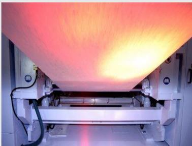
The world's largest spunlaid spinning system – from Oerlikon Neumag – produces non-woven textiles up to 7 meters (23 feet) wide.
