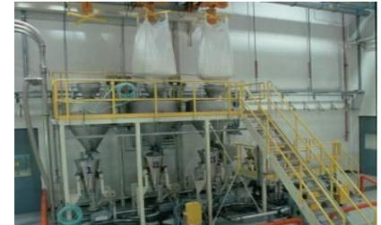
Airlaid lines are for the production of absorbent core materials, wipes, napkins and table tops.
