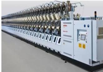
Twisting and cabling machines for high performance yarns in tires and different technical applications
