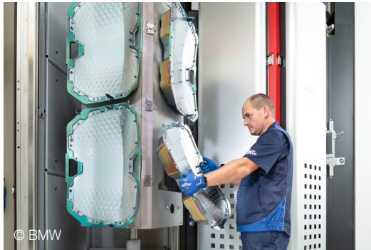
An operator at the BMW factory in Landshut loads the INUBIA B15 with kidneys from the BMW iX.
