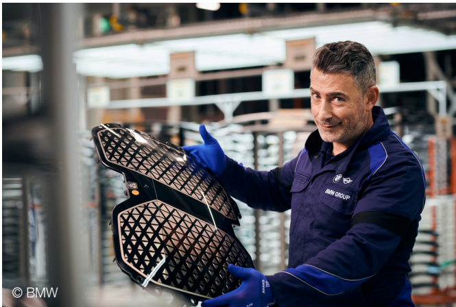
The metallized coating of the kidney of the electric BMW iX enables the integration of sensors, for example to measure the distance to the vehicle in front.
