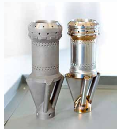
Burner front for gas turbines: AM and conventional design
