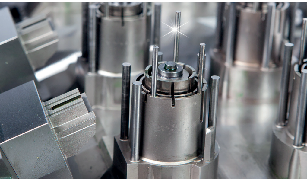
Oerlikon Balzers' new BALINIT MOLDENA for injection moulding and extrusion of filled polymers provides superior abrasion and corrosion resistance for applications with glass fibre reinforced plastics (GFRPs) and fully recycled materials while ensuring a longer mould service life and delivering high-quality products (Picture: iStock)
