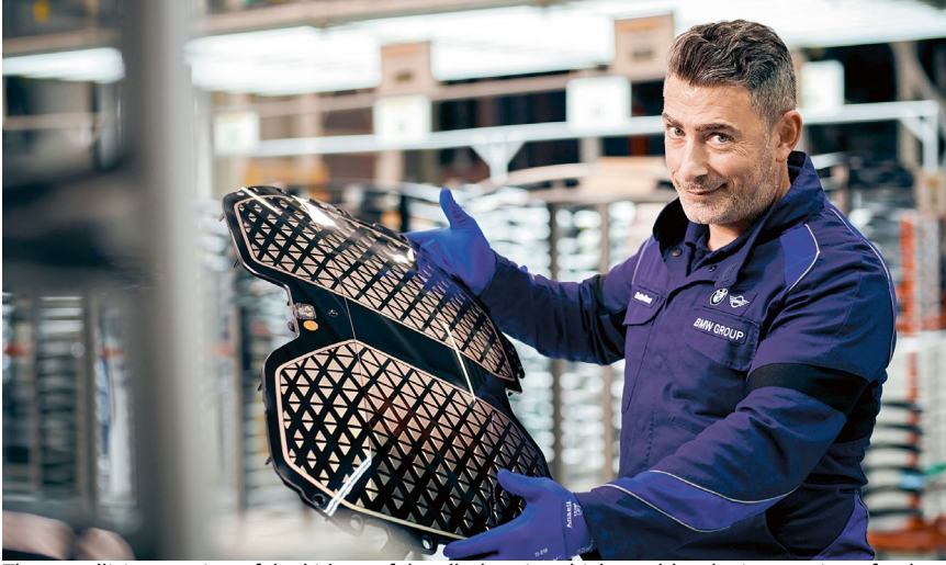
The metallizing coating of the kidney of the all-electric vehicle enables the integration of radar sensors to measure the distance to the vehicle in front.
