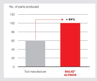
ToolDCMT11T308WorkpieceSteel 1.4837, GX40CrNiSi25-12,<br/>turbocharger componentCutting<br/>parameters $v_c = 110 \text{ m/min}$ <br/> $f_t = 0.40 \text{ mm}$ SourceAutomotive end customer
