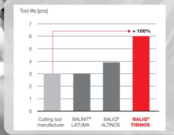
BALIQ TISINOS – milling of nickel based alloy in the power generation and gas turbine industry
