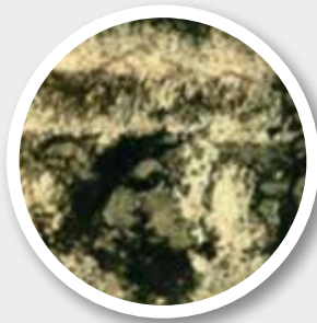
Wear track (30x) of nitrided ring, exhibits heavy galling after 150 m sliding distance
