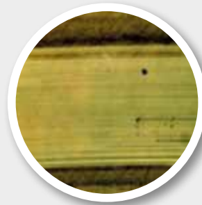
Wear track (30x) of BALINIT® C coated ring exhibits only slight running in (wear depth approx 0.2 \mu m) after 2000 m sliding distance
