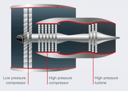
clearance, the more efficient the turbine. Efficiency increases as high as 3 percent are possible here.
