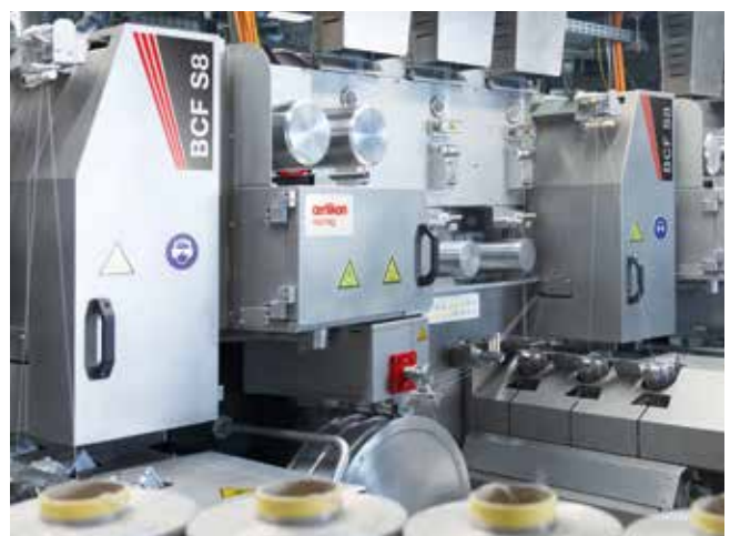
The two core technologies for the Egyptian market: the BCF S8 (bottom) and the eAFK Evo texturing machine.
