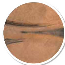
Considerably reduced wear to the thrust pad after 24 hours of operation using the new contacting device with deactivated thrust pad rotation
