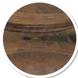
Signs of wear to the thrust pad after 24 hours of operation using the old contacting device with deactivated thrust pad rotation
